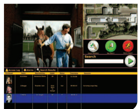
Virtual Turnstile used to verify persons entering racecourse stables. The Ipsotek analytics are able to filter out horses and other objects such as wheel barrows but verifies all persons as having an appropriate RFID pass.
